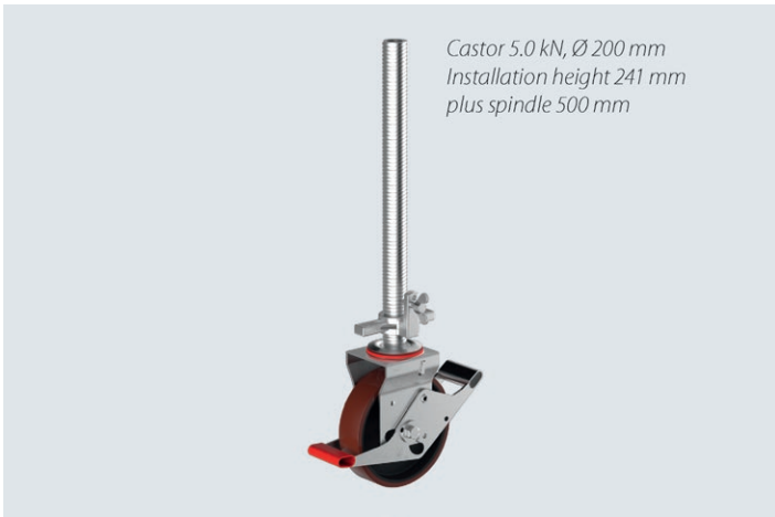
Castor 10.00 kN, Ø 200 mm Installation height: 241 mm plus spindle 500 mm Brake position: 1,000 kg Travel load approx. 400 kg (on level surface)
